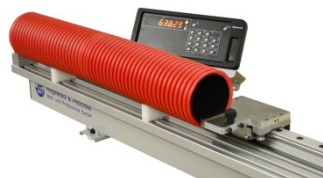
Length measurement on plastic pipes
