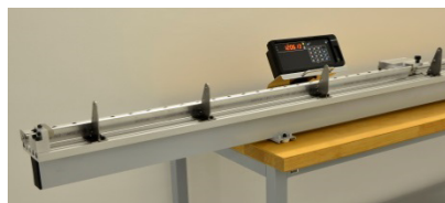
Length measurement on plastic pipes
