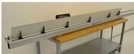
Length measurement on sheet metal strips
