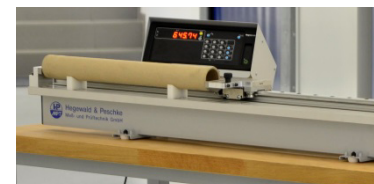
Length measurement on cardboard tubes
